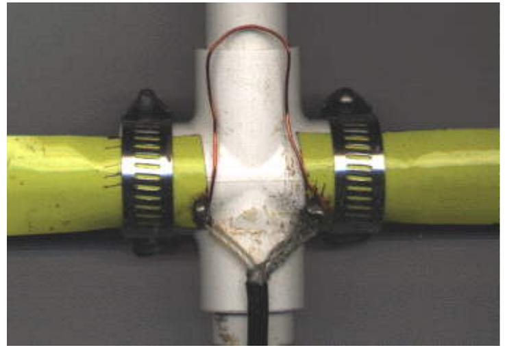
If you wish a slightly neater looking beam, use the self tapping screws. If you do not mind spending a few more dollars for the hose clamps, use them instead. If I were to build another beam I would use screws for the director and reflector, and hose clamps for the driven element. That would give me the best of both methods.
